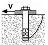
Concrete pry-out failure
