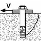
Concrete pry-out failure
