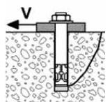
Concrete pry-out failure
