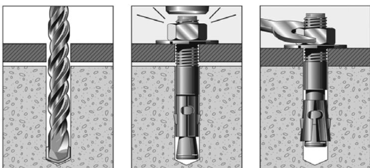
1. Drill the correct diameter hole to the same diameter as the TruBolt™ stud anchor selected.
